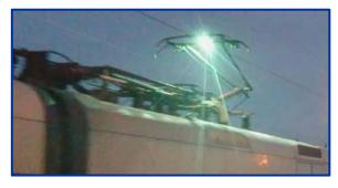
Eliminate costly interruptions of revenue service due to the effect of ice/frost accumulation on the contact wire.
