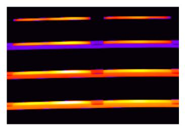
The 3 clips that keeps the circuit on the overhead wire are visible on all pictures.
